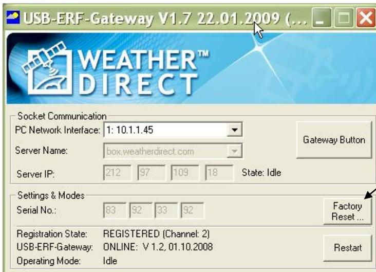
Note: If you do not see the "Welcome" screen (above) and you did not yet register the USB gateway, press the Factory Reset button on the USB-ERF-Gateway software. This will reset the USB gateway and display the serial number it reads inside the gateway. If these numbers do **not** match, use the number in the **Welcome** screen. If the rare case that an unmatched number occurs, please contact Customer Support.
