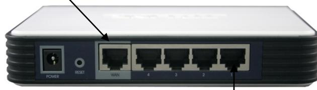
4. Lastly another RJ-45 cat5e network cable plugs into a LAN port on the router at one end, and the other end plugs into your Ethernet → port on the computer (with another one eventually going to the standard gateway).
