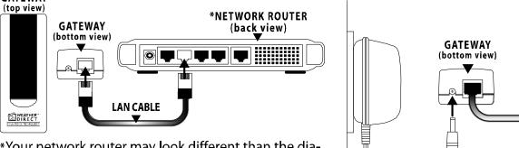
\*Your network router may look different than the diagram. Locate an available port on your router and plug in the included LAN cable. If you do not have a router, please visit www.weatherdirect.com/router
