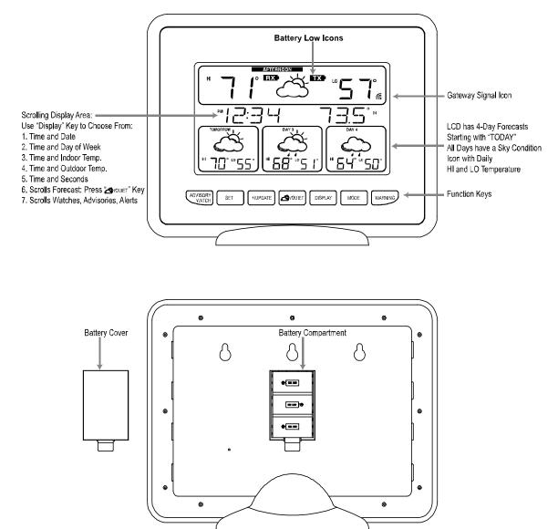
**Note**: If you have any difficulty displaying the outdoor temperature, remove batteries from both the display and the temperature sensor. Let them sit for 10 minutes. Then, making sure the display is in range of the gateway; reinsert batteries first into the temperature sensor, then the display. As the display updates, the temperature sensor will be discovered and connect to the display.
