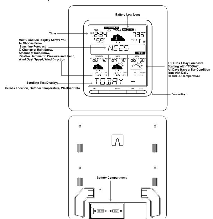
Press the "SNOOZE" Key to cycle through the type of detailed weather information that will display below the forecast icons:
