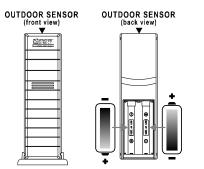
The Outdoor Temperature Sensor uses 2 x "AA", **Alkaline** batteries. To install and replace the batteries, please follow the steps below:
