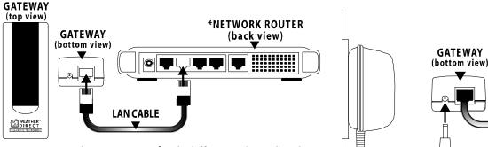
\*Your network router may look different than the diagram. Locate an available port on your router and plug in the included LAN cable. If you do not have a router, please visit www.weatherdirect.com/router
