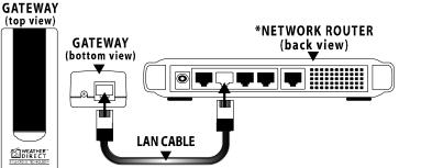
\*Your network router may look different than the diagram. Locate an available port on your router and plug in the included LAN cable. If you do not have a router, please visit www.weatherdirect.com/router
