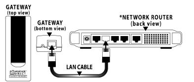
\*Your network router may look different than the diagram. Locate an available port on your router and plug in the included LAN cable. If you do not have a router, please visit www.weatherdirect.com/router
