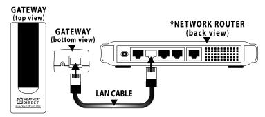
\*Your network router may look different than the diagram. Locate an available port on your router and plug in the included LAN cable. If you do not have a router, please visit www.weatherdirect.com/router
