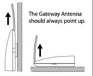
The Gateway should be installed indoors in an easy-toreach location. Registration requires that you press the gray button on the Gateway. It can be mounted securely to the wall with the included mounting plate and drywall anchors.
